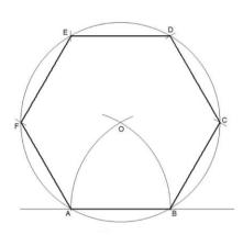
(Hint: On a base line AB cut arcs equally with 30 mm and draw a circle with center O and radius OA, cut arcs equally on the circle, join all points.).
