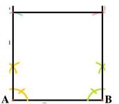
(Hint: Construct perpendiculars from points A and B, take equal measurement of 40 mm and cut arcs to get a square).
