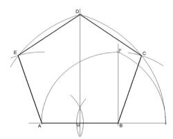
(Hint: Construct a regular pentagon on a base line AB = 30 mm, using compass)
